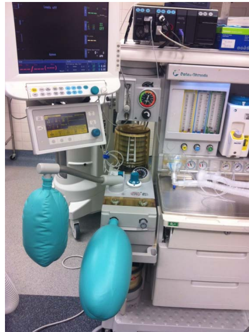
Figure 3. Illustration of a wrinkled bag; here, the bag at the bag mount site has wrinkles, indicating expiratory valve incompetence.
