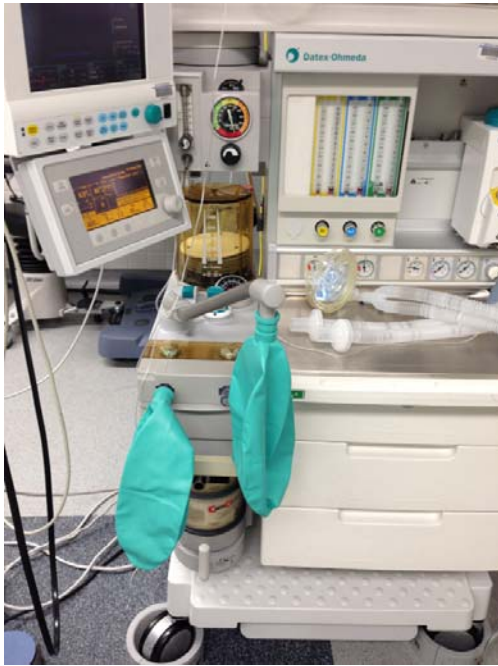
Figure 1. Illustration of the first step of the MPDM; place an extra bag on the inspiratory port.
